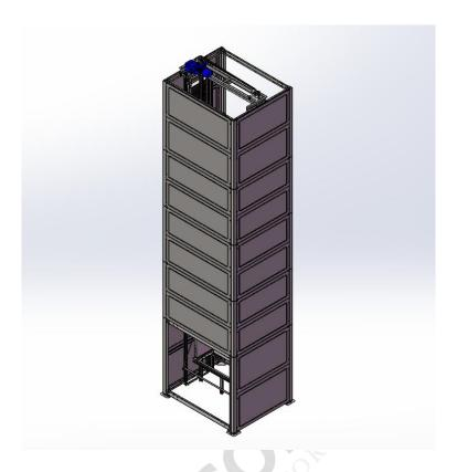
The working principle of a reciprocating lift conveyor involves the drive unit driving the chain through sprockets. The ends of the chain are connected to the load platform and counterweight components respectively. The upward and downward movement of the load platform is achieved by reversing the motor.
