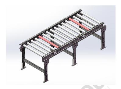
• Roller: Multi-V belt roller with φ50\*1.5mm dimensions, with maintenance-free deep groove ball bearings at both ends, and the roller body made of galvanized carbon steel.
