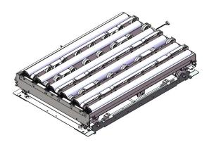
An embedded transfer conveyor is employed to change the direction of movement of packages from roller conveyors by 90 degrees, acting as a lifting and transferring device. Typically, it remains in a low position. When goods are conveyed onto the transfer conveyor, sensors detect their presence, prompting the transfer conveyor to elevate above the conveyor, transferring the goods to adjacent conveyors. Once the goods are delivered, the transfer conveyor descends back to its low position.
