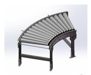
• Roller: Multi-V belt roller with φ50\*1.5mm dimensions, with maintenance-free deep groove ball bearings at both ends, the roller body made of galvanized carbon steel, and externally covered with hard plastic cone sleeves.
